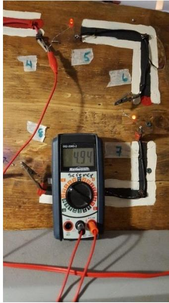
Students can be asked to come up and make those measurements. Voltage drops can be made if the negative test lead from the voltmeter is left permanently on the negative terminal of the power supply. The positive lead from the voltmeter can then be touched at each site and the voltage drop recorded. This is a more telling story than measuring individual drops at each load.
