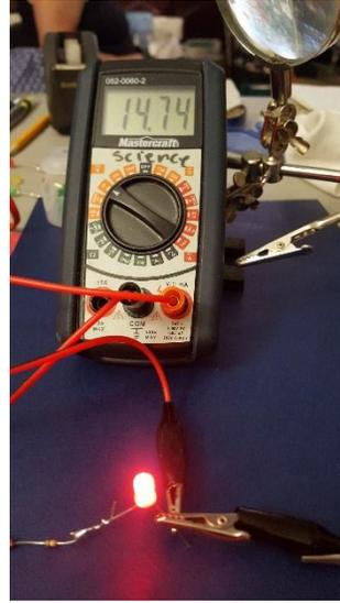
**Part Three: Permanent Display Boards:** Self standing display boards showing series and parallel circuits can be made and sites can be labelled where voltage and current are to be measured. Using alligator clip connections, the circuit can be broken apart to measure current.
