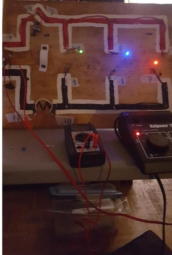
With the initial use of modelling to demonstrate the properties of circuits, the use of low cost LEDs and load resistors, and the creation of permanent displays that employ predictions and measurement, students will acquire the knowledge and skills required in electricity. AS the displays are permanent, and the loads are reliable, the planning and preparation time required will be greatly reduced.
